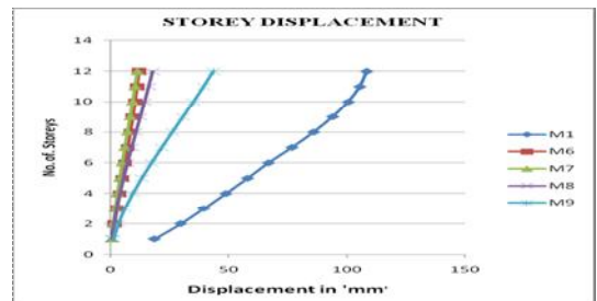
Fig. 24: Storey displacement for CSW
