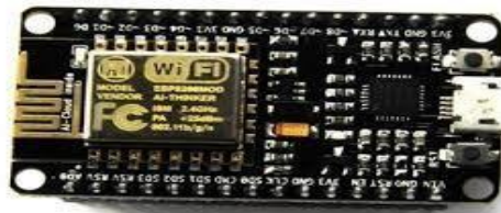
Figure 5: Wi-Fi module (ESP8266 NODEMCU)
