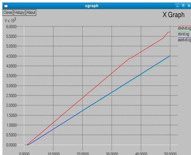
Figure 4 Numbers of Dropped Packets Versus Simulation Time for Random Waypoint Mobility Model
