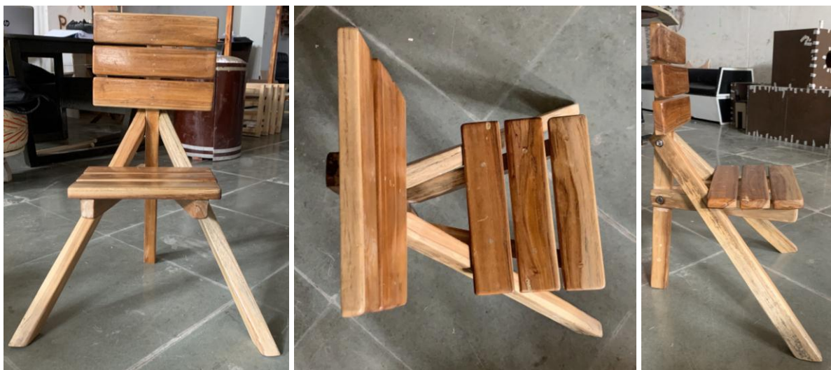
Figure 12: Final 1:1 scale prototype made up of teak wood.
