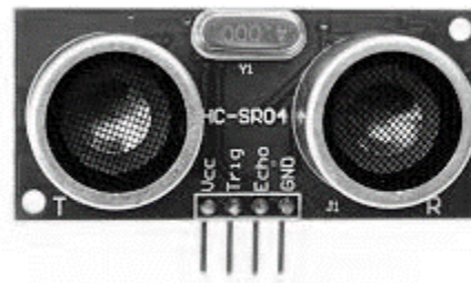
Fig 4:- ultrasonic sensor pin layout
