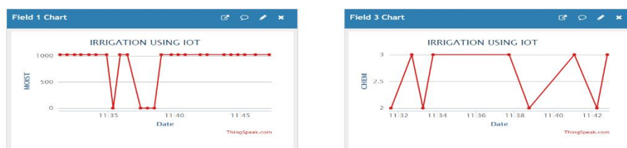
Fig21. Moisture sensor analytics and Smoke sensor analytics
