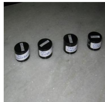
Fig 7. Vicker's Hardness Friction Stir Welded specimens
