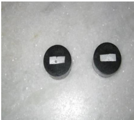
Fig 5. Vicker's Hardness Gas Welded specimens
