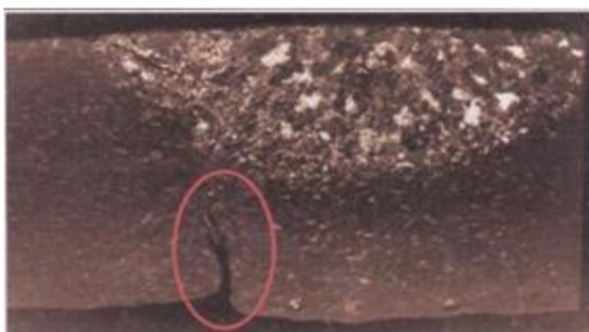
Fig 10. Microstructure of Similar Gas welded specimens
