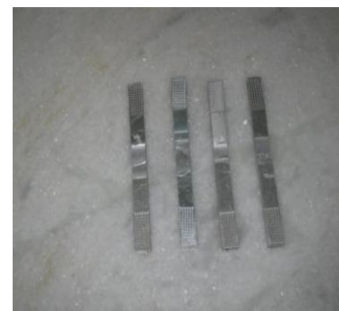
Fig 6. Tensile Test Specimen of Friction Stir Welded specimens
