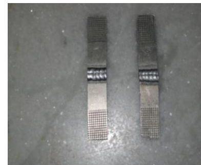
Fig 2. Tensile Test Specimens of TIG Welded specimens
