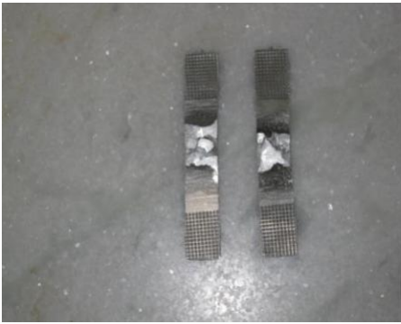
Fig 4. Tensile Test Specimens of Gas Welded Specimens
