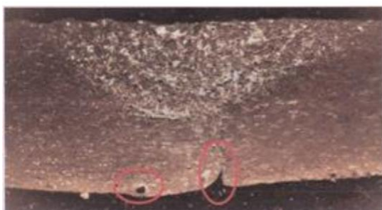
Fig 11. Microstructure of Dissimilar Gas welded specimens
