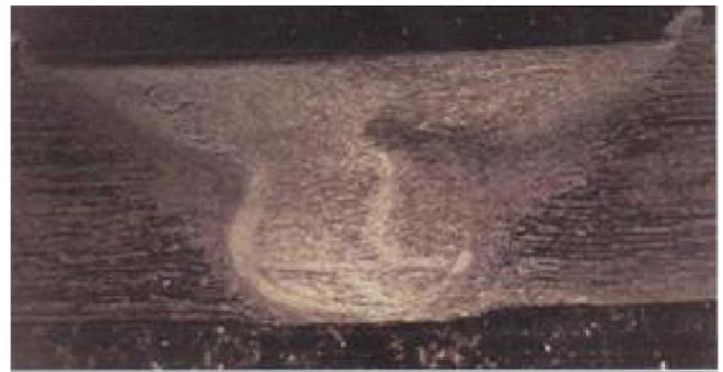
Fig 12. Microstructure of Similar FSW welded specimens
