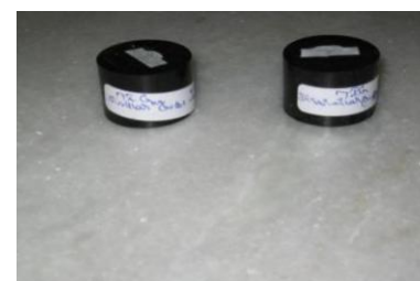
Fig 3. Vicker's Hardness TIG welded Specimens
