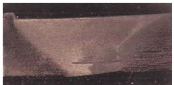
Fig 15. Microstructure of Dissimilar FSW welded specimens
