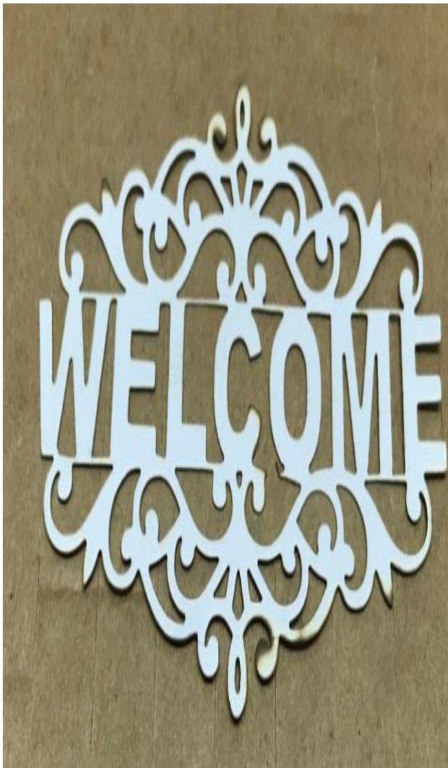
Fig. 6 Laser Cutting of Welcome Sign Using Wi-Fi Module
